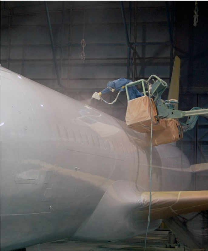
CRYOCLEAN® CO 2 snow pre-cleaning for painting and coating processes
