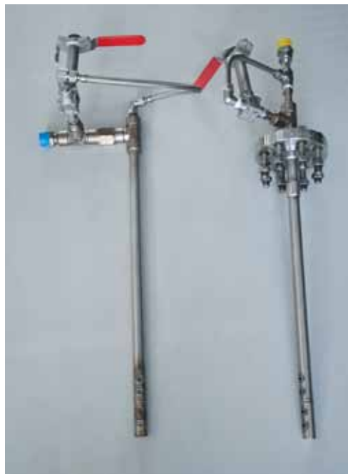
Figure 18: Nozzles for injecting liquid nitrogen into a gas stream [4]
