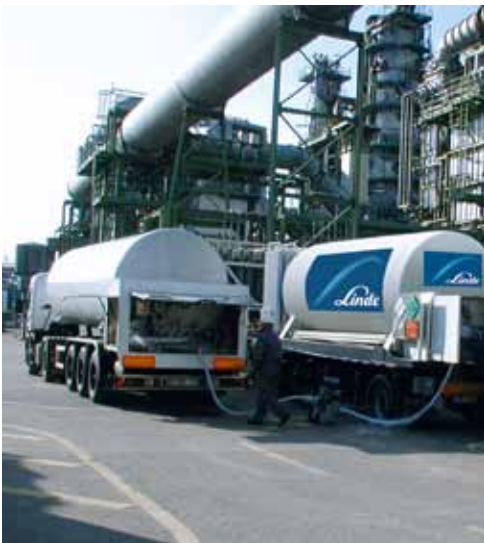
Figure 28: Use of liquid nitrogen to cool down a reactor
