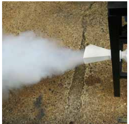
Figure 14: Special nozzle for vaporising carbon dioxide [4]
