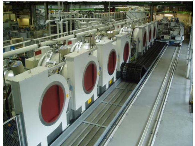
Figure 5. A modular vacuum carburising system at BMW (photo courtesy of ALD)
