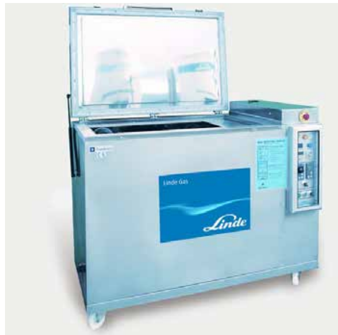
Figure 4. A top loading cryogenic treatment box
