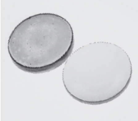
Fig. 4 – Damaged laser optic
