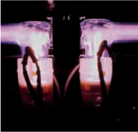
Fig. 1 – Excitation of laser gas in a laser resonator
