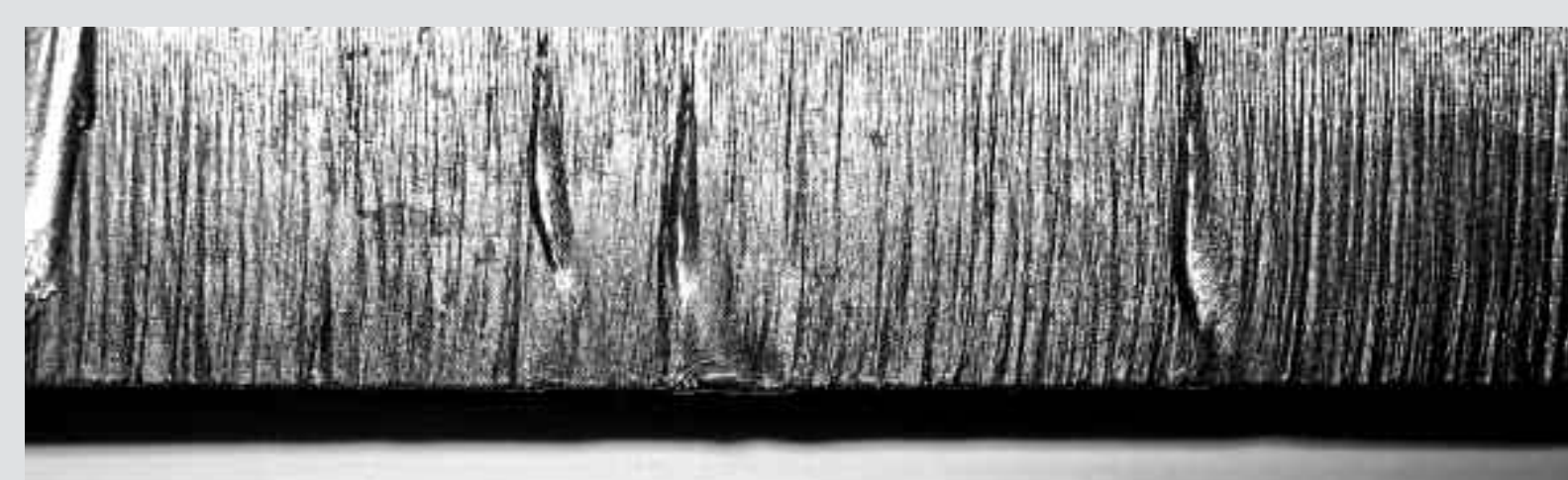
Example of how material quality can affect cut quality - oxygen cutting of low-grade mild steel.
