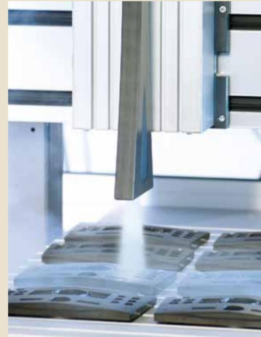
Thanks to varying blasting geometries, it is possible to clean large and also very small surfaces, either completely or partially, and coat them afterwards.
