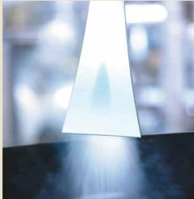
CRYOCLEAN® snow is based on a fundamentally new functional principle. By feeding liquid CO<sub>2</sub> (LIC) into a specially designed device, particularly solid snow particles are produced and "shot" immediately onto the surface with compressed air. The system is designed for medium-power cleaning processes and a layer thickness up to approximately 1 mm.
