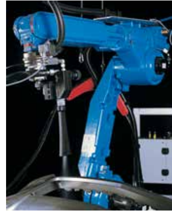
Automated cleaning of plastic parts with CRYOCLEAN® snow
