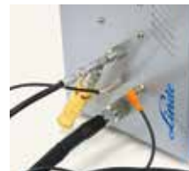
Supply connectors and additional grounding
