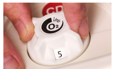
2.3 Turn the flow selector to 5 lpm and check that gas flows through the firtree for at least 5 seconds. Return the flow selector to zero.
