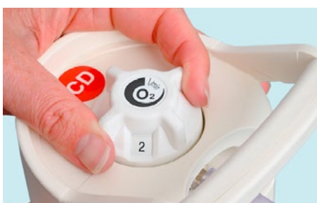
2.1 Turn the flow selector to 5 lpm and allow any gas in the regulator to vent. Return the flow selector to zero when you hear the gas stop flowing.
