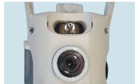
1.3 Check the outlets appear clean and free from any damage.
