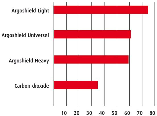
The addition of carbon dioxide and oxygen to argon for MIG welding carbon steels increases weld fluidity – allowing faster welding speed and improving the stability of metal transfer.
