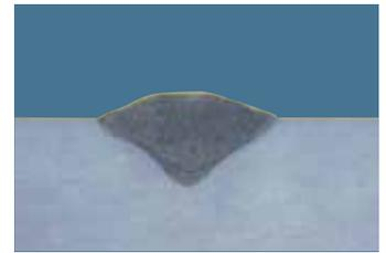
The addition of helium to the shielding gas results in a hotter welding arc than that produced from pure argon.
